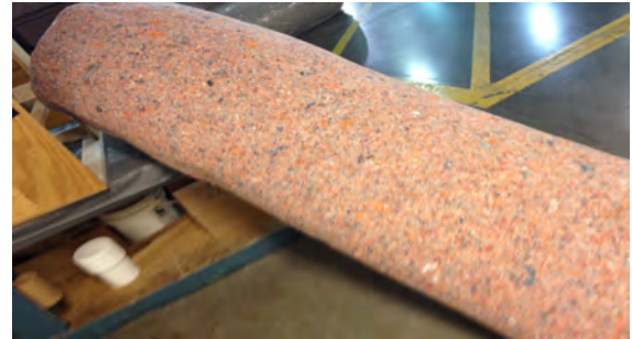
Padding, made from recycled inmate clothing, used in Arizona Correctional Industries spring mattress production.
